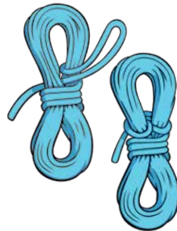
gasket hitch – secures a coil of rope for storage.
