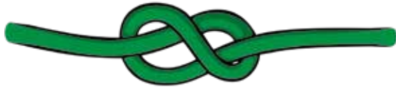
Figure 8 knot – Typically used as a stopper knot to avoid having an end of the rope pull through a knot, such as the end of the climber’s line.
