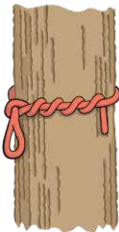
timber hitch – commonly used to secure a fixed eye sling as an anchor, usually with a minimum of 5 tucks.
