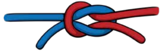
square knot – used to join two ropes of equal diameter.
