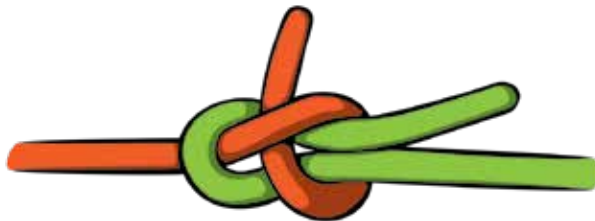
sheet bend – used to attach two lines together, particularly when they are different sizes. The sheet bend can be used to attach a rigging line to the climber’s line to send it up to the climber. The slipped sheet bend is a variation that is easy to untie.
