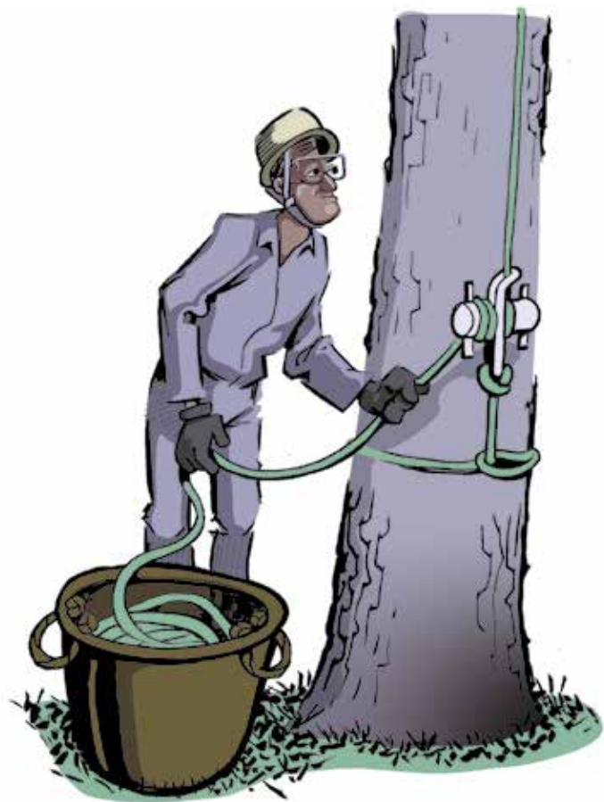
Using a barrel to keep rigging lines "clean".
